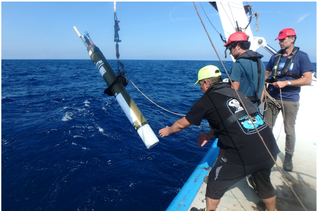
Deployment of a profiling float equipped with a pCO 2 sensor at the vicinity of the BOUSSOLE site.
